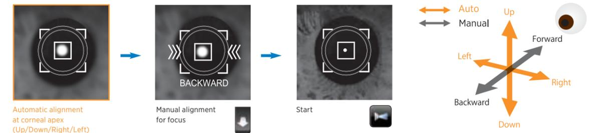
The difference between the pupil center and the corneal apex, allows the CT-1 / CT-1P to easily take measurements.
